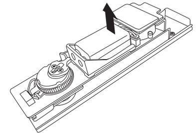
5. Slide back the key assembly alarm kit.
