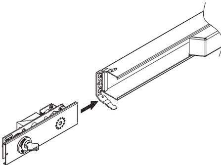
6. Make sure to line it up with the groove of the push rail assembly.
