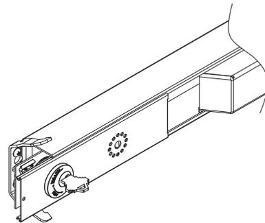
7. Carefully pry back the mounting brackets to its original position.
