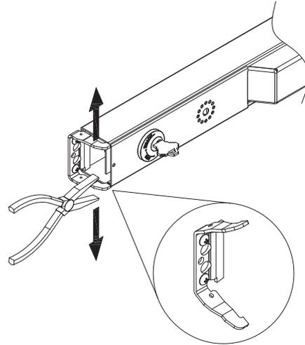
3. Slide the key assembly towards the edge of the exit device.
