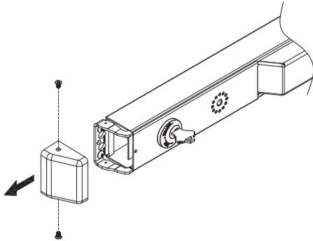
2. Slightly pry both sides of mounting bracket as shown.
